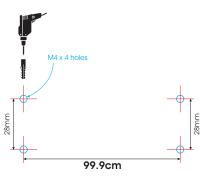
**b.** Drilling holes example with **LUMITUBE IP68-26.3W-133.5cm**
